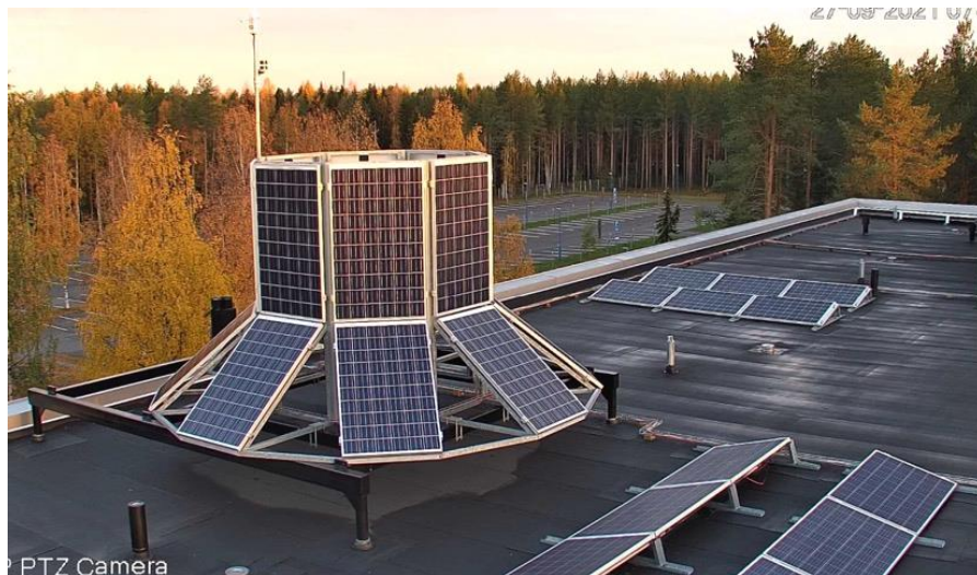
Fig 15: Experimental carousel setup on the roof of University of Oulu
