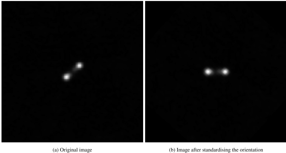
Figure 1. Results of applying the rotational standardization algorithm, which leads to a 41.68^\circ clockwise rotation.
