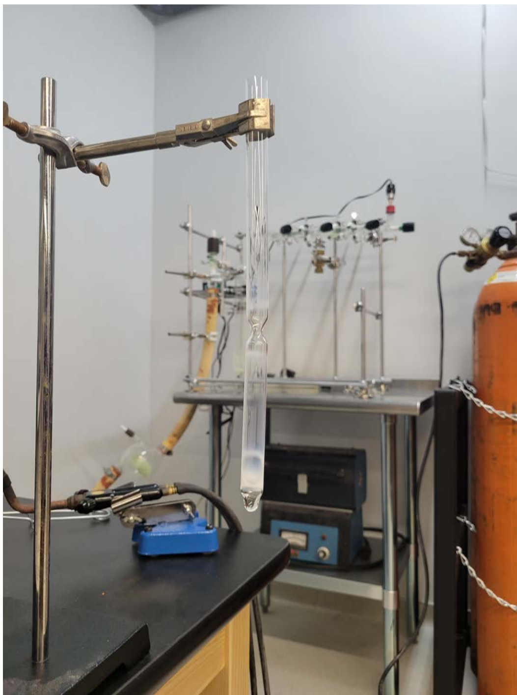
Fig. 4.2: The quartz tube before powder insertion. One end of the tube is sealed. Then, approximately 10 cm above the sealed end, the tube is heated for necking to occur.
