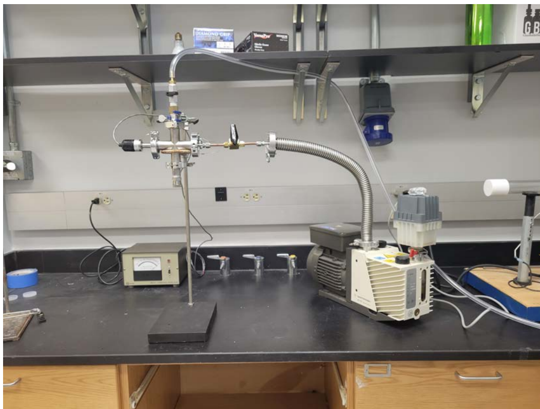
Fig. 4.6: Setup for the vacuum sealing process.
