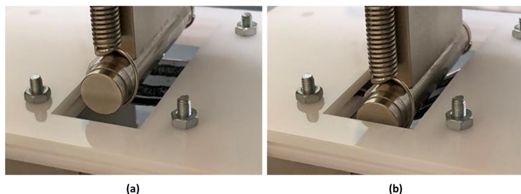
Figure 3. Bending tests with an applied force of 6.6 N, (a) press and (b) release motion.
