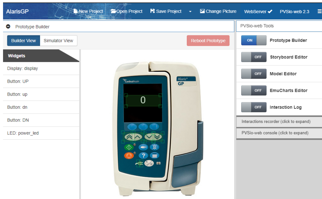
Figure 2.8: Prototyping environment of the PVSio-Web. Green areas over the prototype image represent the widgets depicted on the left panel. The right panel lists all the available environments of this tool.
