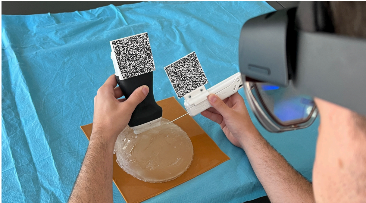
Figure 16: Third-person usability test view of a user performing the biopsy in a breast phantom.
