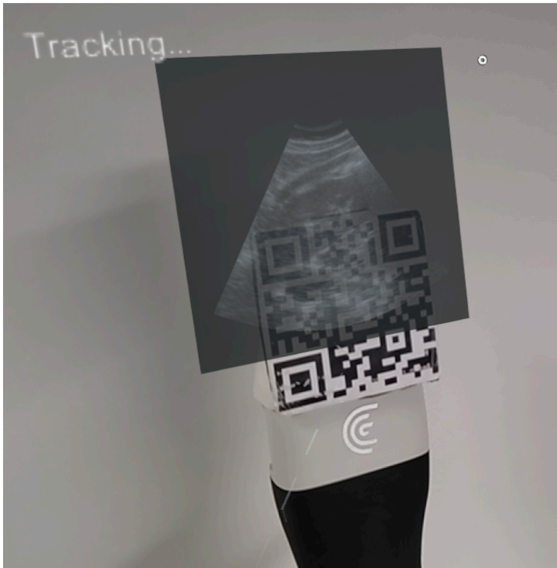
Figure 9: View from HoloLens display showing the US image over the QR code assembled at the top of the portable US probe.
