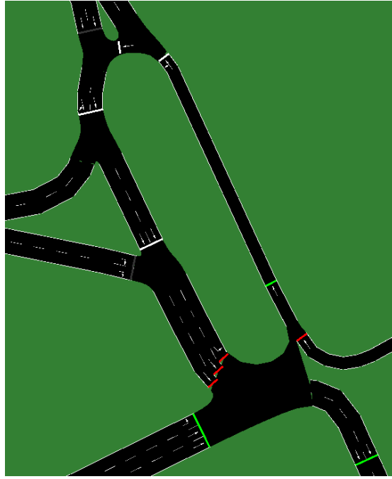
Fig. 3. SUMO network converted from OpenStreetMap: after corrections.
