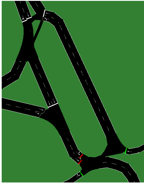
Fig. 2. SUMO network converted from OpenStreetMap: before corrections.
