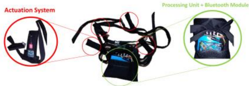
Figure 3. System developed, illustrating the main components and interfaces between them.
