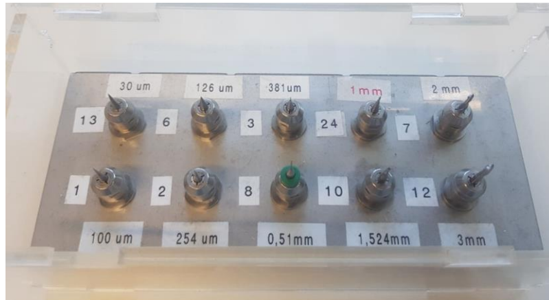
Figure 19 - Tools used in micromilling of the company Zecha.
