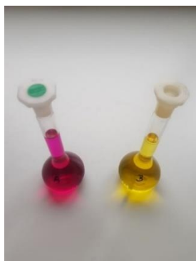
Figure 47 - Solutions A and B with phenol red in 500 mL volumetric balloon.
