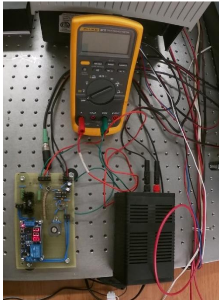
Figure 10 Timer device connected to the computer, spectrophotometer, and ammeter.
