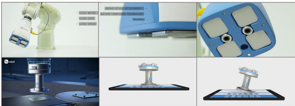
Figure 2.7 – Two examples of gripper solutions exploiting the gecko-like adhesion surface. The images on the right, demonstrate the release methods. The griper on the top image releases the surface by contracting its pads. The griper on the bottom as two ways of releasing: like it's exhibited in the picture, by tilting the gripper, or by clapping the piece in a fixture and moving the gripper ( OnRobot , n.d.).
