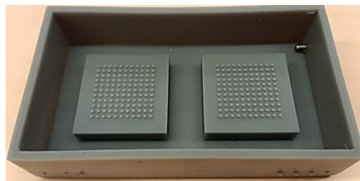
Figure 4.6 – Printed mold in 3D printer SLA.
