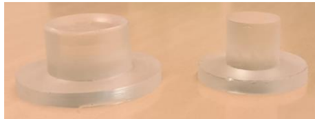
Figure 5.19 – Flat samples fabricated with the same contact area as the structures A and B.
