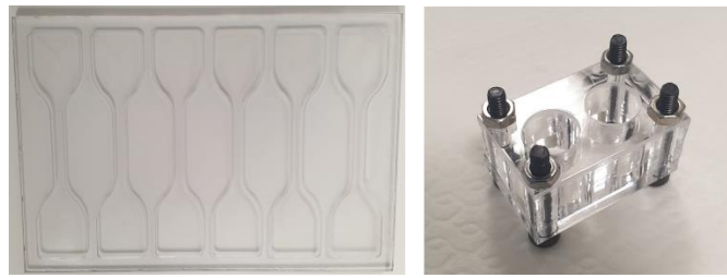
Figure 4.2 – Tensile (left) and compression (right) negative molds.
