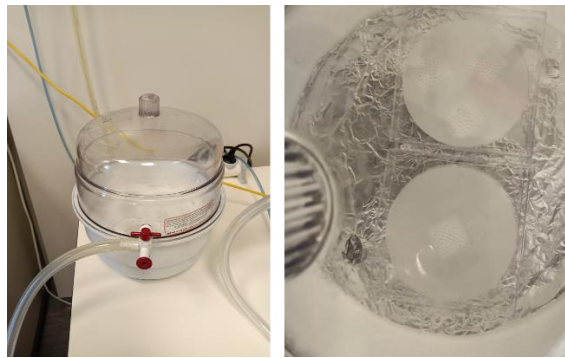
Figure 4.7 – Degassing of air in a vacuum desiccator.
