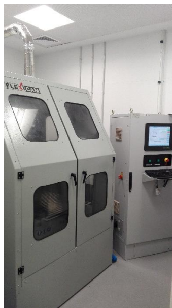
Figure 3.3 – CNC (3 axis tool) FlexiCam Viper , allows the machining of pieces with size up to 650x650x280 mm, and has a fixed gantry (moving table design for maximum stiffness and high accelerations).
