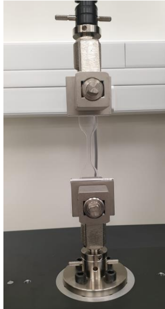
Figure 3.9 – Tensile testing of PDMS specimen.
