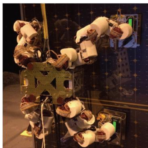
Figure 2.9 – LEMUR 3 climbing on a mock-solar panel surface using gecko adhesive grippers (Parness et al., 2017).
