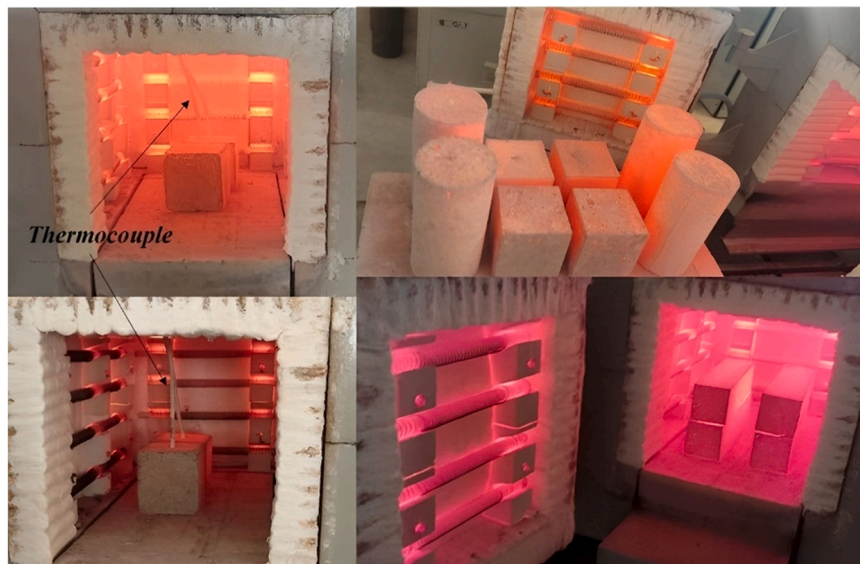
Fig. 1. Heating of concrete samples in the furnace.
