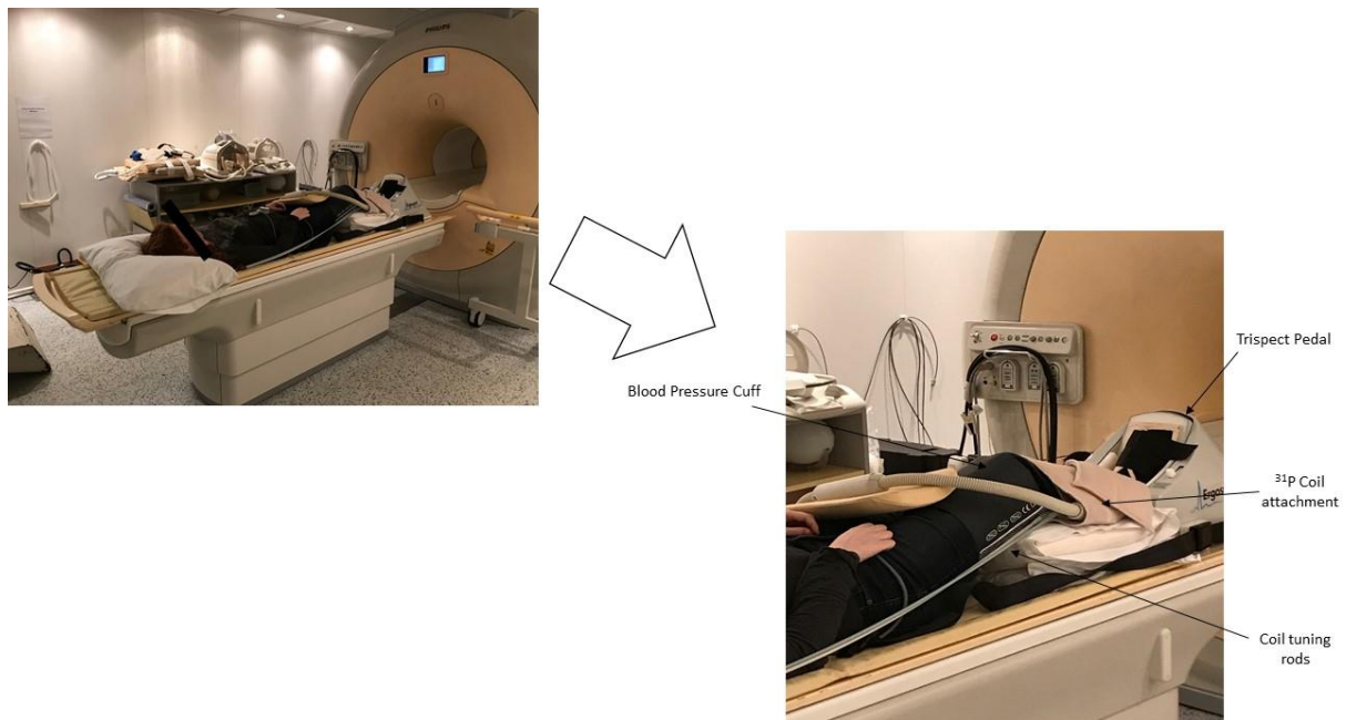
Figure 3-13. Experimental Trispect set-up for ^{31}\text{P} MRS experiments on the Philips Achieva.
