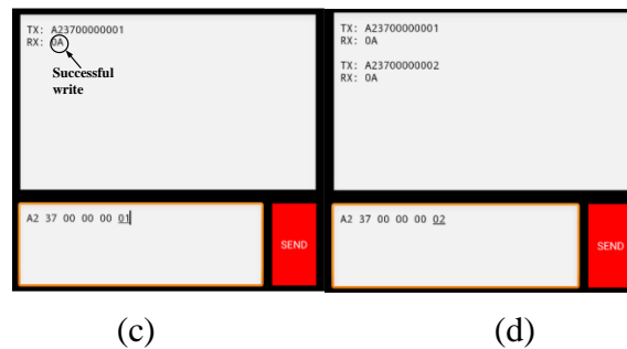
Fig. 8. Screen shots of NFC Shell in use, where (a) shows the command, address and data to be sent. In (b) the screen presented before coupling to a tag. (c) shows a successful write of flash pattern 01 to the tag and (d) similarly shows the same for pattern 02.
