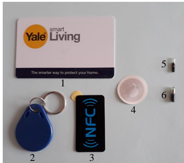
Fig. 1. A selection of planar type NFC tags (1-4). Implantable glass animal tags (5 and 6).
