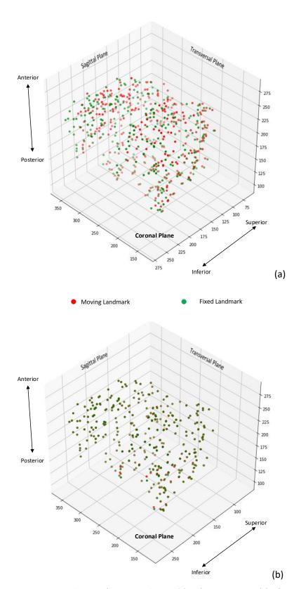
Figure 6.3:Annotated points of DIR-LAB, volume 8. (a): Before registration, (b): After registration, all axes in millimeters. The more color-saturated points represent points closer to the viewer.
