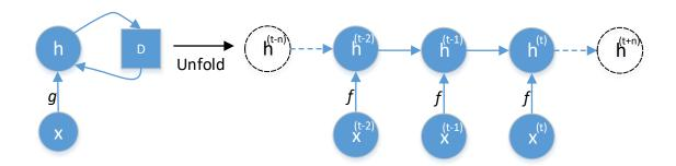
Figure 3.9: Recurrent Neural Network. Left is an RNN diagram with a delay unit (D). Right, it's an unfolded representation of the network.
