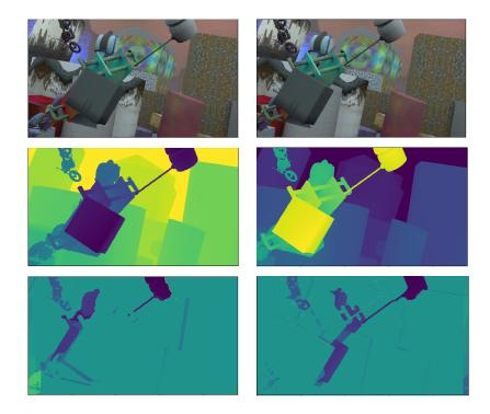
Figure 2.15: FlyingThig3D Dataset. Top stereo: image pairs (Mayer, et al., 2016). Middle: Disparities of the left image (negative values) and the right image. Down: occlusion of the left and right images, respectively. Clearly, in the occlusion areas, the pixels within this area have no correspondence.
