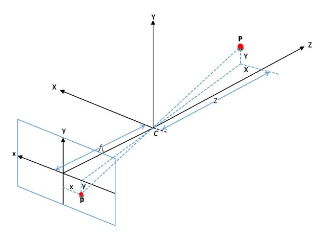
Figure 2.1: Graphical representation of the pinhole (or perspective projection) camera model (Wang, et al., 2002), C is the camera optical center (i.e., pinhole), f is the focal length.
