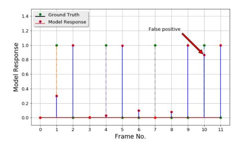
Figure 4.19: Evaluating a double blink in the model's response. On consecutive blinks, the model produces false positive.
