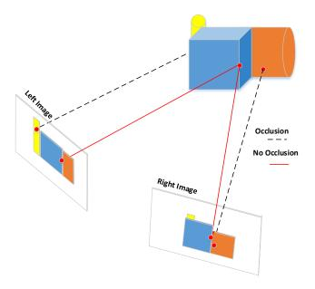
Figure 2.13: Object Occlusions. The orange cylinder on the right is shown wider in the right image while smaller on the left image. In the other case, the yellow cylinder is entirely shown on the left image while it disappears on the right image and only shows on top of the blue object.
