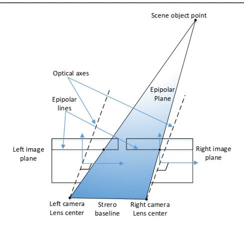
Figure 2.8: Binocular stereo geometry
