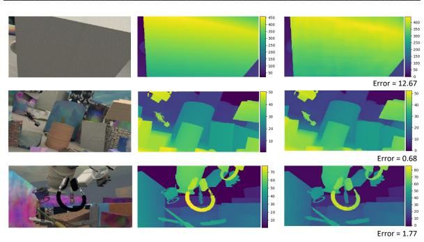
Figure 5.7: Disparity model qualitative test with FlyingThings3D. A sample result from the fourth experiment - the FlyingThings3D dataset. (Left): Left image, (Middle): The corresponding disparity maps ground truths, (Right): The estimated disparity maps using unsupervised training. Under each estimated disparity map, the error with respect to the GT is reported.
