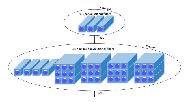
Figure 3.4: An example of a Fire module in the squeeze Net.
