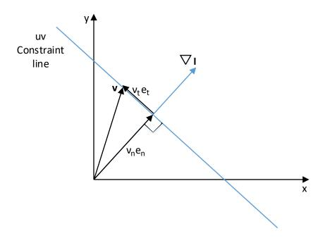
Figure 2.6: uv constraint line. The motion vector ( $\mathbf{v}$ ) decomposition into normal ( $v_n e_n$ ) and the tangent ( $v_t e_t$ ) components. Any tangent component can satisfy the optical flow equation for given  $\nabla I$  and  $I_t$ .
