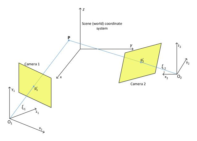
Figure 2.3: Camera motion with a static scene or stereo vison (Change shape pinhole to be behind the image plane) (Tekalp, 2015).
