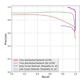
Figure 4.10: The network performance of Figure (8) tested on the Eyeblink8 dataset. The high performance obtained with time distributed CNN with LSTM layers.
