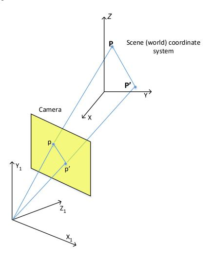
Figure 2.4: Projection of the 3D scene motion vector onto the image plane.
