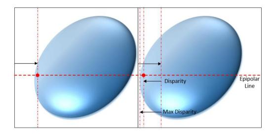
Figure 2.12: Disparity Estimation in binocular image set. The Max Disparity represents the maximum searching space for the disparity algorithm to find the disparity value.
