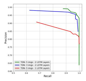
Figure 4.11: The networks performance of Figure 4.9(c) tested on the Eyeblink8 dataset. The highest performance is obtained with Time Distributed Network with two LSTM layers when the input has five frames. The network performed less when the input is three frames or when one LSTM layer is used.
