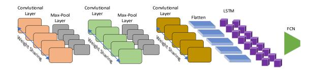
Figure (App.C) shows a Time-Distributed Convolutional Neural Network with an LSTM example.
