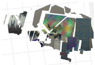
Figure 2.16:3D Scene Reconstruction. Using the disparity estimation in companion with the camera specification to reconstruct the 3D scene from single image, the left image obtained from FlyingThings3D dataset (Mayer, et al., 2016).
