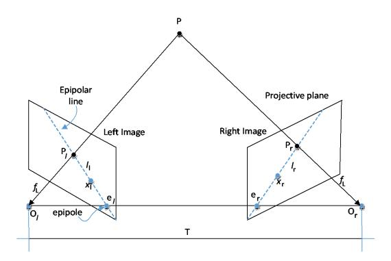
Figure 2.11: Converged binocular camera setup.
