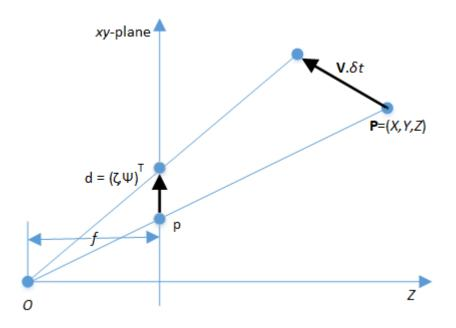
Figure 2.17: Displacement Field
