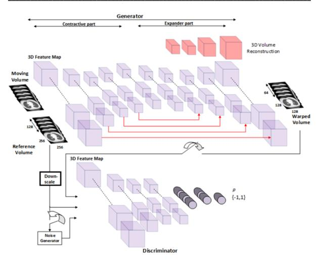
Figure 6.1: A simplified diagram representing the proposed network architecture. It consists of two parts: the contractive-expander as the generator and the discriminator.
