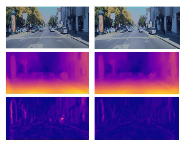
Figure 5.5: Consistency Feature Map. Top: stereo image pair, Middle: Forward and Backward disparities, Bottom: Consistency Feature Map shows the area where the occlusion appears as a hot area.
