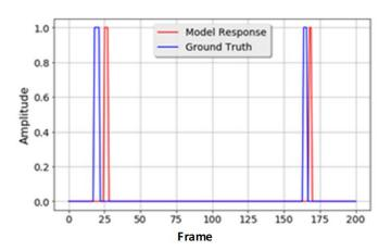
Figure 4.14: Model response to the input from the Talking Face dataset. The response of the model lags by a few frames. As the video buffer receives the targeted blink sequence, including the eyelid transition, it responds within a range of 2 to 5-frame delays. During the evaluation, this delay is considered a correct response and compensated for during the performance estimation.
