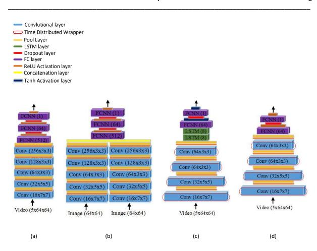
Figure 4.9: Suggested models for Eyeblink Detections. a) Early fusion with five frames instead of 2. b) Late fusion (Karpathy, et al., 2014). (c) Proposed network time-distributed convolutional network with LSTM, (d) The same network as in (c) but without LSTM.
