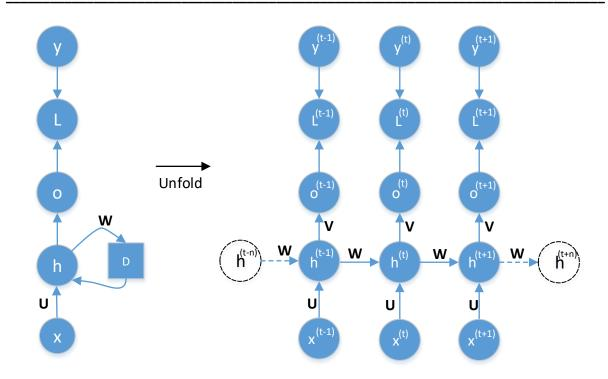
Figure 3.10: Recurrent Neural Network Equivalent Circuit. The model maps the input sequence 'x' to its corresponding output 'o'. The loss function L compare between the model output o and the ground truth y.
