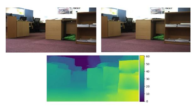
Figure 5.8: Disparity model qualitative test with different camera settings. Disparity Estimation for stereo image with stereo camera of 12cm baseline and 3.8mm focal length.
