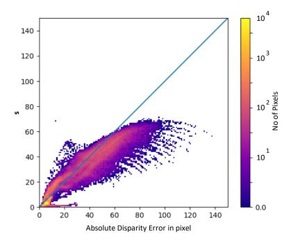
Figure 5.11: Dual channels absolute error uncertainty test. Absolute error uncertainty relation on the Kitti dataset for dual channel model. The logarithmic colour scale encodes the number of pixels having the respective error and estimated standard deviation  $\sigma$ . In case of optimal uncertainty estimation, all pixels should be aligned as close as possible to the diagonal line
