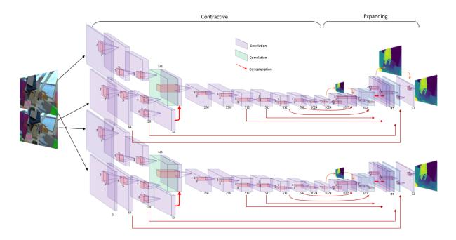
Figure 5.3: Proposed disparity estimation CNN model. The network reported in (Mayer, et al., 2016) (Odena, et al., 2016) has been duplicated to perform parallel channels. One channel produces the backward disparity feature while the other channel predicts the forward disparity features. Each layer of these channels has been set with weight sharing accepts the correlation layer since it contains no weights.
