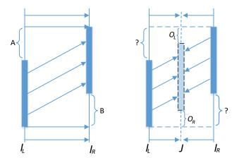
Figure 2.14: Occlusion detection. To render a new image, J from the left and the right image information from A and B areas need to be available to reconstruct the OL and OR areas. It is impossible to do that without incorporating the two disparity maps (Ince & Konrad, 2008).
