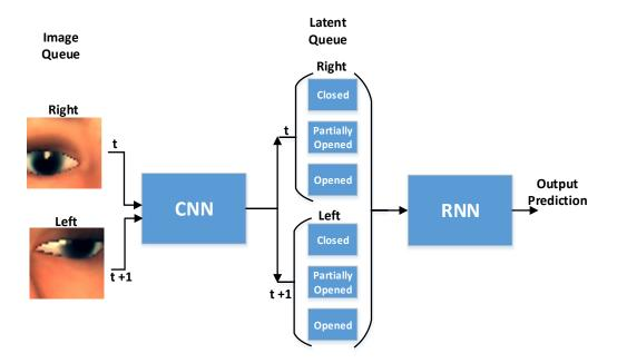
Figure 4.5: The CNN-RNN processing pipeline diagram.
