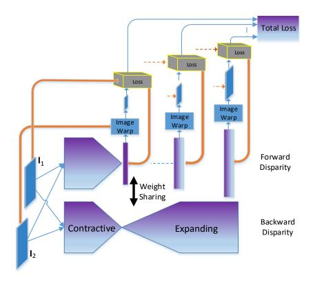
Figure 5.4: The details of the warping module in the proposed network. The same arrangement that is shown on the upper side of the network is also available on the lower side of the network, and it is not shown.
