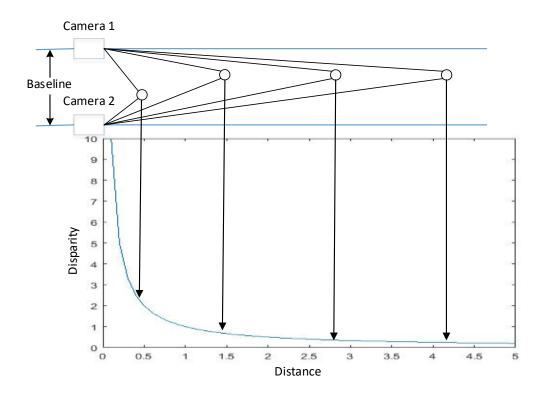
Figure 2.10: Disparity-Depth relationship in parallel image plane setup of Figure 2.9.
