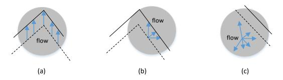
Figure 2.7: The effect of the area structure on the optical flow estimation. (a) no aperture problem with moving corners (spatially distributed structure). (b) The case of moving edge where the local neighborhood of all the gradients are parallel. In this case, the estimation of the optical flow in ambiguous. (c) in the case of a textureless surface, the constraint becomes completely inapplicable (Szeliski, 2011).
