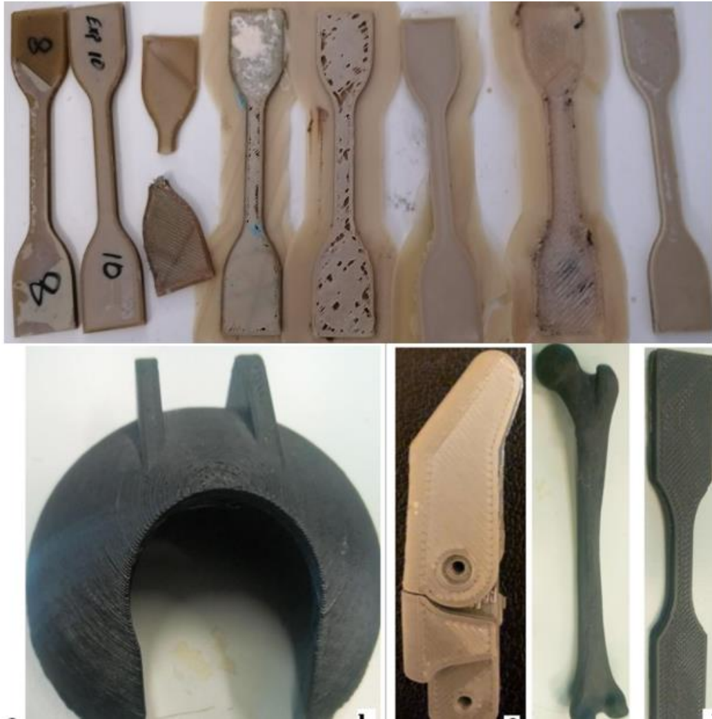
Figure 4.15 Different printing Scaffold and Nozzle 0.2-0.4 of the different bone implants.
