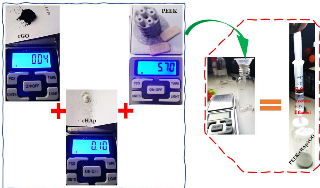
Figure 4.3 Fabrications of composite by cold modification of PEEK scaffold.
