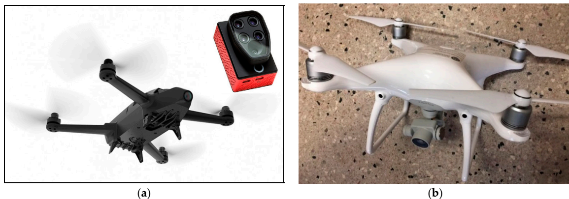
Figure 2. (a) Parrot Bluegrass quadcopter with Parrot Sequoia sensor; (b) DJI Phantom 4 Pro quadcopter with stock RGB camera.
