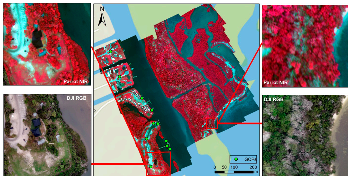
Figure 7. Orthomosaic and geo-referenced UAV products at 0.25 m spatial resolution using the near infrared false color combination. Two enlarged areas show both false color images from the Parrot Bluegrass and nature color image from the DJI Phantom 4 Pro.
