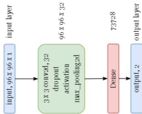
Figure 17: Shallow CNN Structure
