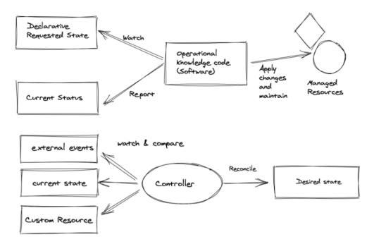
Figure 3: Operator and Custom Controller [13]
