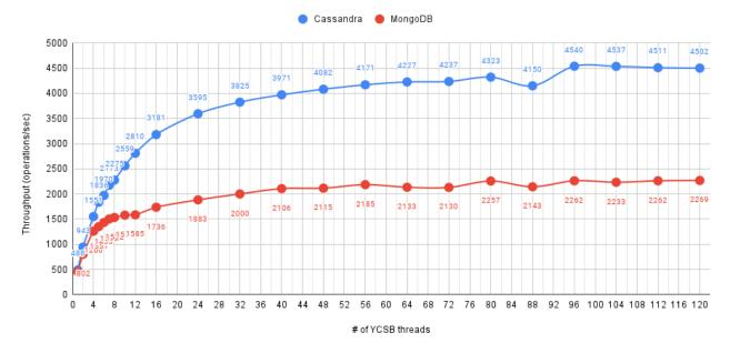
WorkloadC: Read Only - Throughput vs Threads
