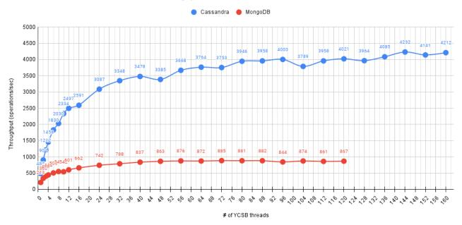
WorkloadA: 50% Read, 50% Write - Throughput vs Threads
