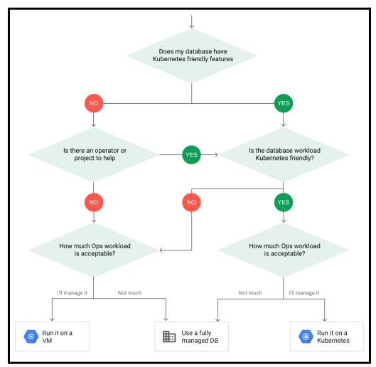
Figure 4: To run or not to run a database in K8s [4]
