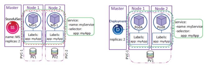
Figure 2: Difference between StatefulSet (left) and Deployment (right) [6]
