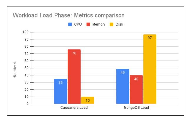
Figure 9: Metrics comparison during load phase
