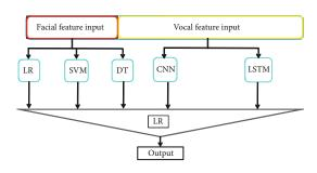
FIGURE 1: FV-Stacking architecture.
