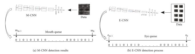
FIGURE 9: The process for obtaining the closure state of the mouth and eyes.
