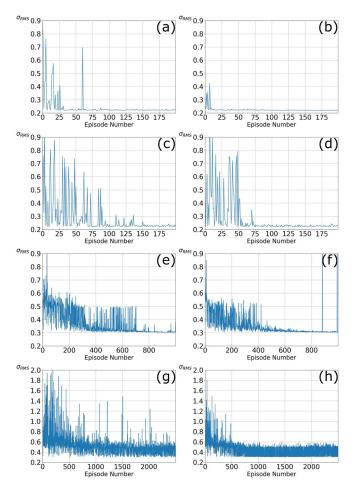
FIG. 17. (Color online) The lowest  $\sigma_{RMS}$  discovered per episode during training. These are results by varying the algorithms used, number of scatterers, and use of gradient assisted inverse design.
