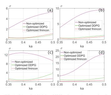
FIG. 11. (Color online) Variation of TSCS vs ka comparing suppression of curves for M = 6, 8, 10, and 12 rigid scatterers following the procedure described in Sec. II C for DDPG at a larger number of scatterers and using a reward function defined by Eq. (13).
