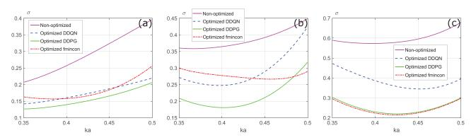
FIG. 7. (Color online) Variation of TSCS vs *ka* comparing suppression of curves for M = 2, 3, and 4 scatterers for thin nickel shells. For configuration of M = 2 and 3 thin nickel shells, DDPG surpasses *fmincon* and performs better at the range of wavenumbers at which the configurations are optimized and beyond this range.
