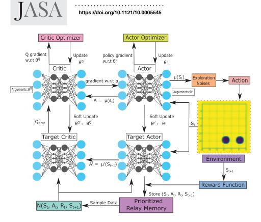
FIG. 3. (Color online) Diagram of DDPG agent interacting with the environment by adjusting cylinder position.
