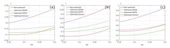
FIG. 8. (Color online) Optimized TSCS vs ka results comparing elastic titanium thin shells for M = 2, 3, and 4 scatterers. All optimized configurations exhibit a final suppressed TSCS response. For configuration of M = 4 thin titanium shells, DDPG outperforms *finincon* within and beyond the range of wave-numbers at which the structure is optimized.
