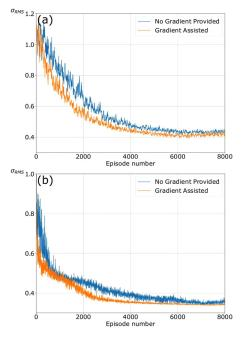
FIG. 4. (Color online) Performance of DDQN (a) and DDPG (b) with and without gradient provided in the state vector for M = 4 rigid scatterers.
