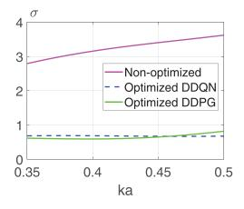
FIG. 14. (Color online) TSCS against normalized wavenumber ka for initial, DDQN, and DDPG optimized configurations of M = 20 rigid cylinders of radii  $a_j$ , where  $ka = k_{\max}(a_j)$  and j = 1, ..., M.
