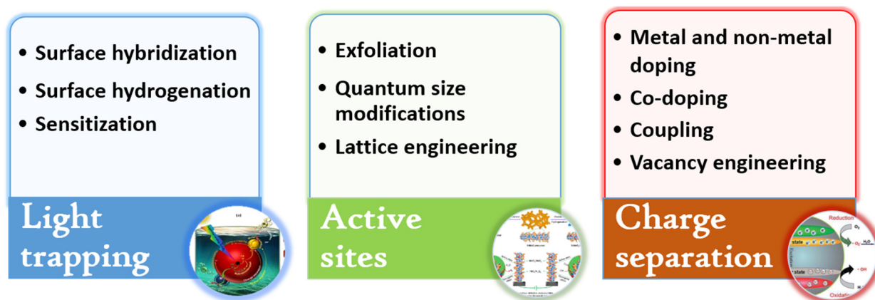
Figure 3. Types of chemical modifications in TiO 2 .
