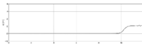
Figure 8. Time series of the water level at the top of the technical pier (gauge wg11).
