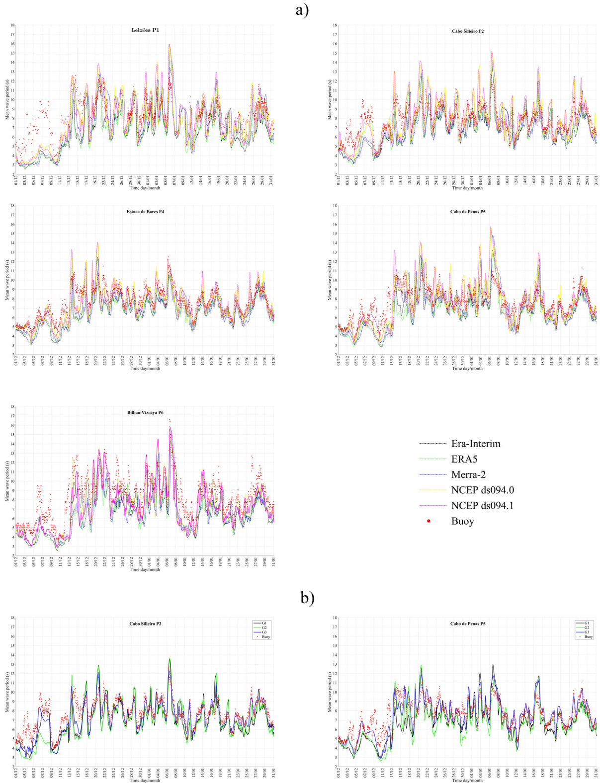
Figure 4. Measured and modelled Tm02 for the period between 01.12.13–31.01.14. Red dots represent buoys measurement, dotted lines are SWAN results for each wind dataset considered. The bold line indicates the best fit for each buoy. a) Comparison of measurements and G1 computational grid. b) Measured and modelled results with ERA5 wind data representing all three computational grids, in buoy locations P2 and P5.
