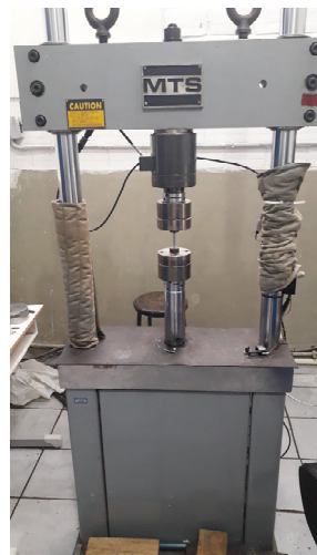
Figure 2. (a) Drawing of the tensile specimens (dimensions in mm). (b) Used MTS 810 servo-hydraulic universal testing machine. (c) One tensile specimen assembled on the testing machine.
