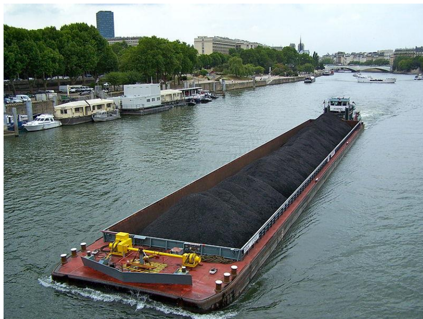
Figure 4.3 Barge transporting soil for land reclamation (Wikimedia Commons, 2011)
