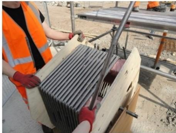
Figure 3.30 Shape array inclinometer (Shape accel arrays, u.d.)
