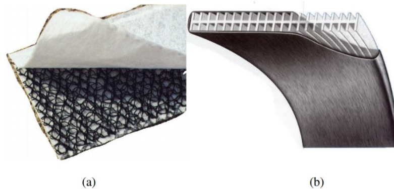
Figure 3.3 Typical types of PVD (a) Colbond drain (b) Mebra drain (Rujikiatkamjorn, 2005)
