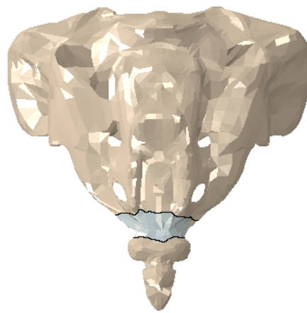
Figure 5.6: Finite element model of the sacrum and coccyx in brown and the sacrococcygeal joint in grey (posterior view)
