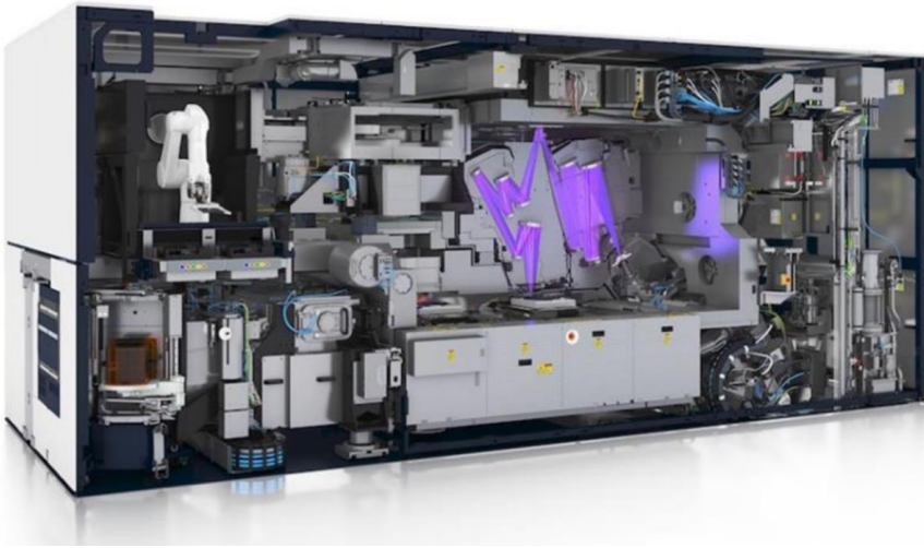
Figure 1.3 Artist impression of an ASML EUV lithography machine. The optical trajectory of the EUV light is highlighted in purple, with the EUV source position on the far right, the reticle in the upper part and the illuminated semiconductor wafer in the center of the picture (Image source: ASML).
