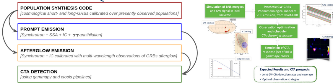
Figure 2: (Left:) Scheme of the GRB consortium publication work. Synthetic spectra and light curves are obtained by a population synthesis code and used to feed the CTA analysis pipeline. (Right:) Workflow for the GW consortium publication. After the simulation of BNS merger, a phenomenological (short) GRB is associated to it. The optimal pointing strategy is then obtained by a dedicated algorithm in order to cover efficiently the sky area of the GW source. Each pointing is then analyzed by means of the CTA analysis pipeline.
