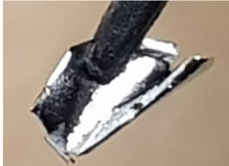
Figure 5.4 Photograph, showing a pair of tweezers (dark object coming in from the top) that holds a freestanding, metallic thin film of \text{Ru}_{77}\text{Mo}_{23} with a thickness of 200 nm, after annealing-induced delamination at 700^\circ\text{C} from the oxidized \text{Si}(100) substrate.
