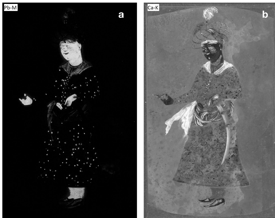
Fig. 17 a MA-XRF elemental distribution map for lead (Pb-M). b MA-XRF elemental distribution map for calcium (Ca-K)
