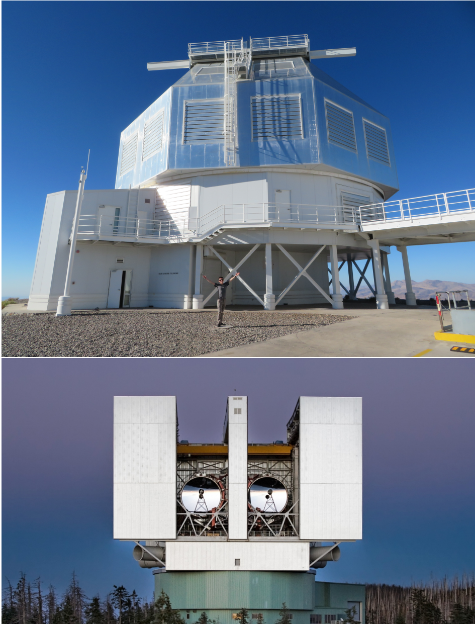
Figure 1.8: The two telescopes used to obtain the observations presented in this thesis. Top panel: The 6.5-m Magellan Clay Telescope at Las Compañas Observatory, Chile, with an exoplanet observer shown for scale. This telescope hosts the MagAO system and a 180^\circ vAPP coronagraph. Image credit: Jayne Birkby. Bottom panel: The Large Binocular Telescope (LBT) at Mount Graham International Observatory, Arizona, USA. The ALES IFS and a dgvAPP360 coronagraph are installed at LBT. Image credit: Large Binocular Telescope Observatory (LBTO), University of Arizona.
