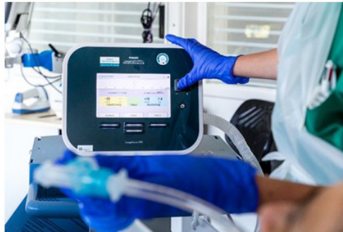
Figure 2. Mechanical insufflation-exsufflation device
