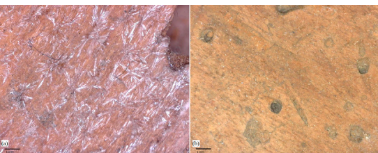
Figure 6. (a) Before and (b) after mechanical removal of the DDT crystals on the wooden surface of the bisj pole. Microscopic photos
