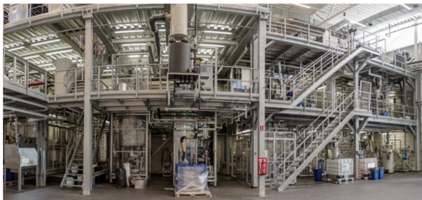
Figure 6. YXY ® Technology pilot plant in Geleen, The Netherlands consisting of an SDH unit for MMF, an oxidation unit for cFDCA and a purification unit to produce pFDCA.
