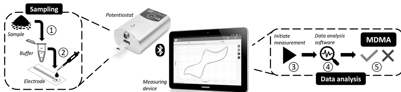
Fig. 1. Sampling and analysis procedure for the electrochemical MDMA sensor.
