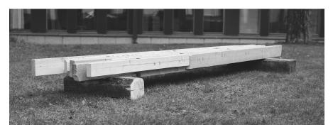
Figure 8. A prototype fabricated for a natural exposure test (before aging).
