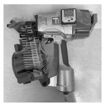
Figure 5. A nail gun (Fasco®), with an angle reader and a spirit level temporarily taped on and compressed beech wooden nails (Lignoloc®) loaded.
