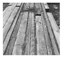
Figure 9. Dirt accumulation on the surface of the pototype structure during the natural exposure test.
