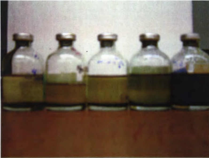
Figure 1. Particle precipitation in four sediment inoculated serum bottles and one uninoculated bottle, all filled with ferric citrate medium and incubated at 30°C for two weeks.
