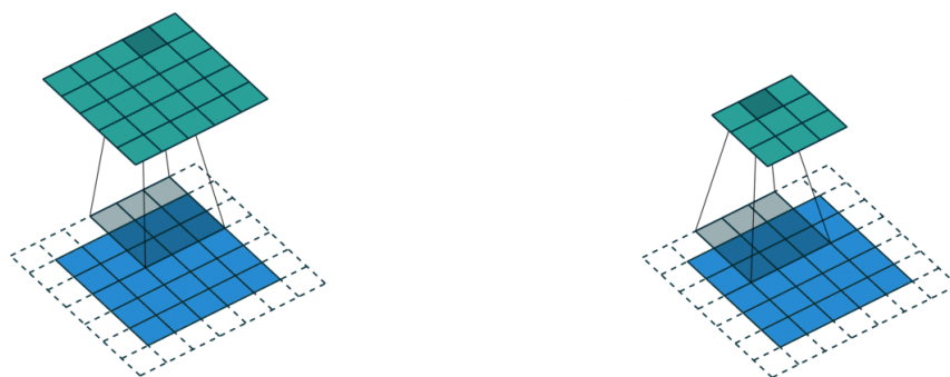
Figure 3.5: Left: Convolutional Layer with a 3x3 filter, padding, and a stride of 1, Right: Convolutional Layer with a 3x3 filter, padding, and a stride of 2 (source: [55])
