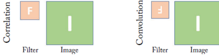
Figure 3.4: Graphical comparison between the correlation operation and convolution operation in signal processing. The CNN convolution is the same as the correlation operation (source: [36])
