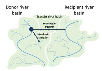
Figure 1: Illustration of donor and recipient basins within Inter- and Intra-Basin Water Transfers. Source: Author's own illustration.
