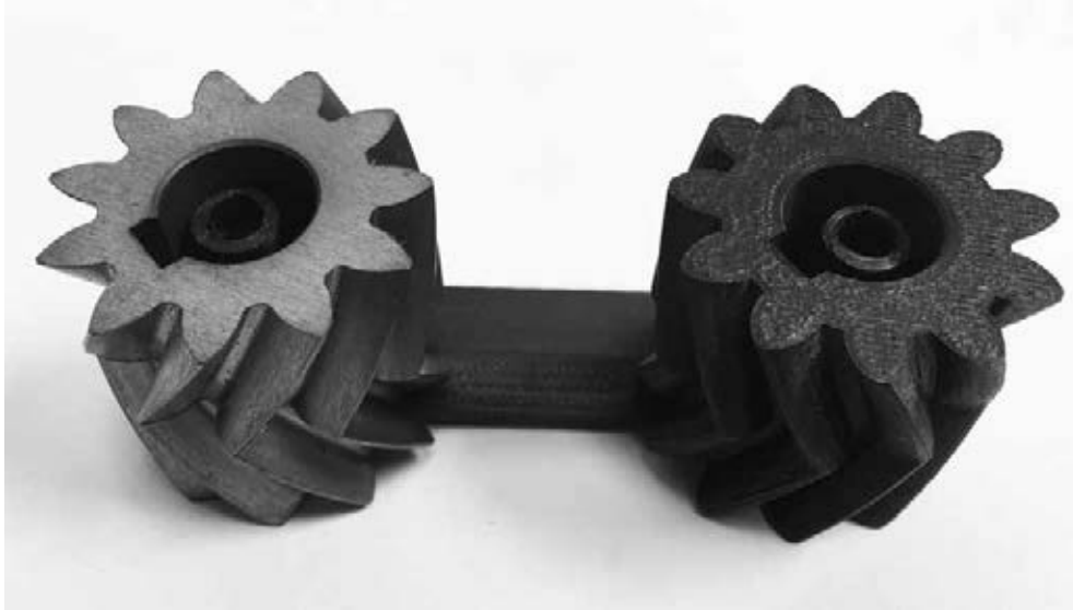
Photo 4. The gear that was redesigned and rebuilt using CAD and 3D printing technology to perform with higher efficiency. Credit: Author.
