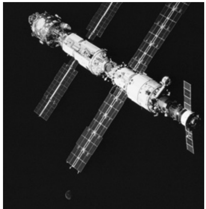
Photo 2. The STS-106 crew members captured this view of the International Space Station (ISS) showing the darkness of space in the background and the multiple PV arrays. The International Space Station makes extensive use of solar arrays to generate electrical energy to maintain the operational status of the ISS, the ongoing experiments, and the crew. (Courtesy of NASA)
