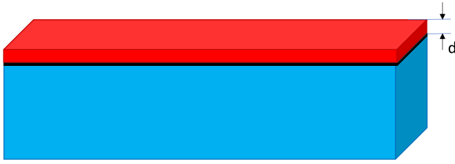
Figure 4. A metallic (N) layer of thickness d (red) coupled by the proximity effect to the bulk superconducting (S) substrate (blue). The black layer between N and S depicts a resistive interface barrier.
