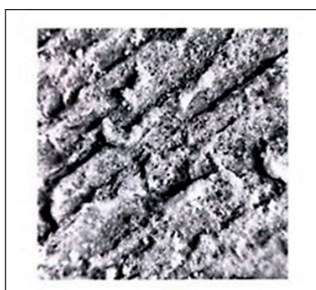
Fig. 1. Photograph of a coated heat exchange surface, namely, a layer of aluminum oxide nanoparticles deposited on a microstructure
