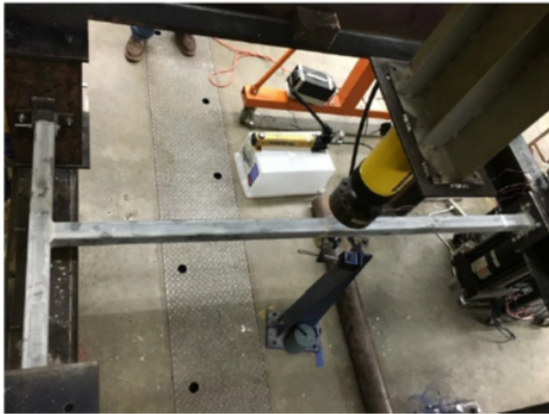
Fig. 2. Sub-assembly setup for quasi-static load test.
