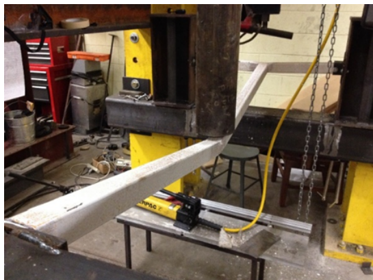
Fig. 3. Sub-assembly setup for impact load test.
