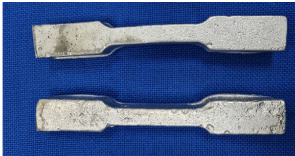
(a) (b) Figure 2. Aluminum Cast Part (a) Before and (b) After Machining
