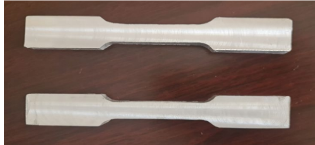
(a) (b) Figure 2. Aluminum Cast Part (a) Before and (b) After Machining
