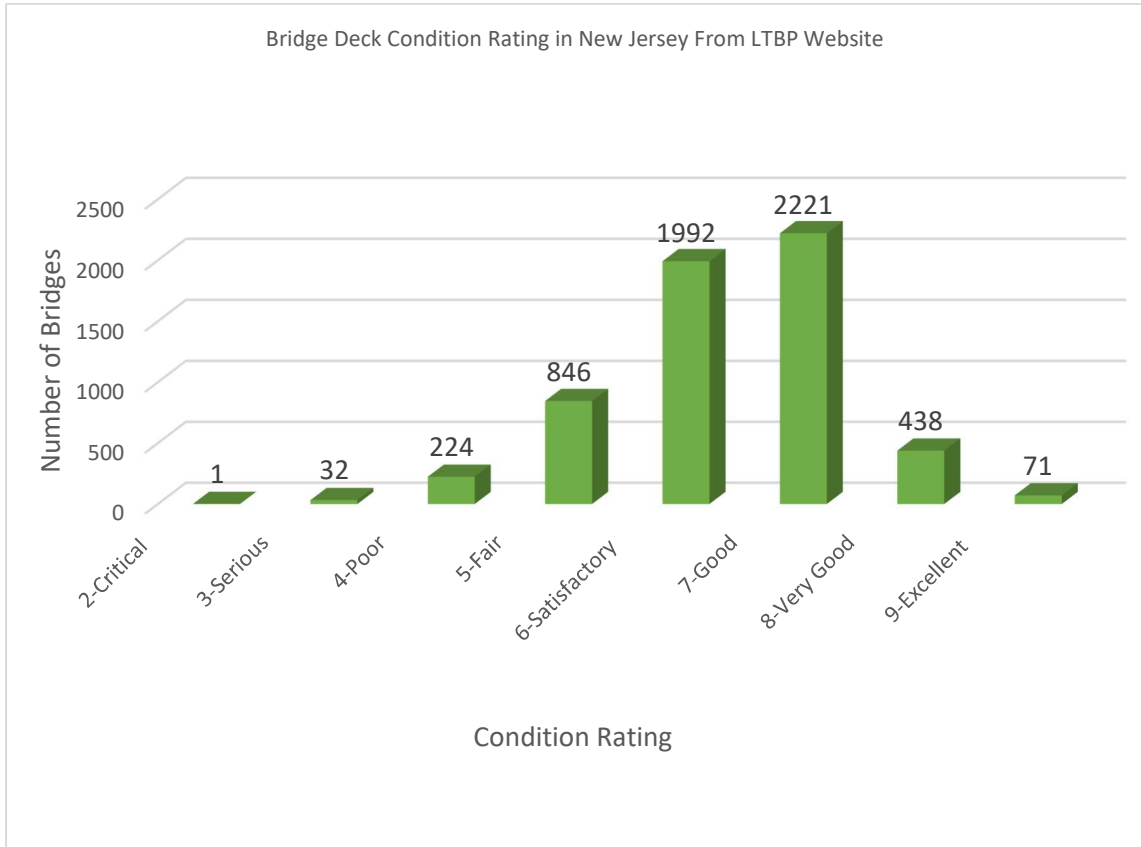
Figure 6. Bridge deck condition ratings for New Jersey from the LTBP website.
