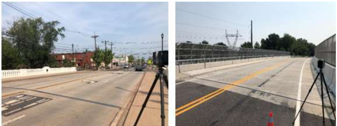
Figure 20. Typical location of scanner: (a) Scanner located on deck's shoulder; (b) Scanner located on the sidewalk.
