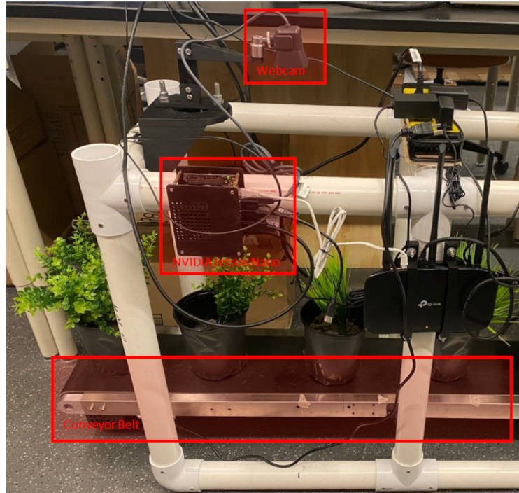
Laboratory Test Setup of the CNN-Based Vision Module
