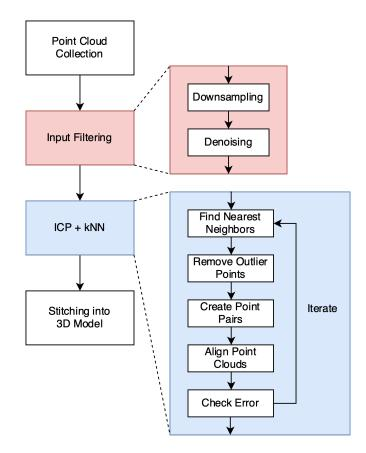
ICP works through two basic steps: First, estimate paired points. This estimation is typically done through a similarity or distance metric. For example, for each point in B, the paired point is the nearest point in A. Using these pairs and a sub-optimal rotation and
