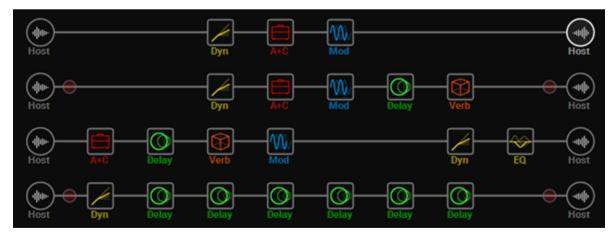
Figure 14 Processing of each string by four timbral lines in GASP system, crossfading into one another at different times.
