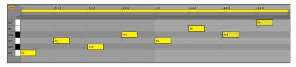
Figure 10 Selection of GASP system's Guitarpeggiator patterns as Ableton Clips. MIDI notes represent on-off switching of TrackGate for arpeggiation effects. Each on-off event corresponds to gate switching for an individual string.
