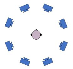
Figure 3 Depiction of an eight-loudspeaker circular array supporting a 2D, 360° spatial representation.
