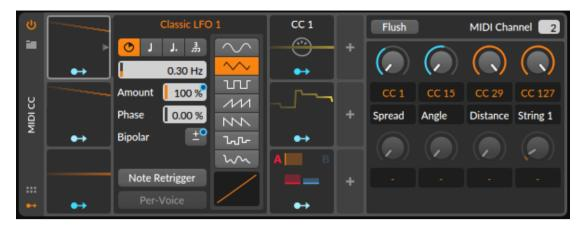
Figure 16 Bitwig's Classic LFO configured for a single string in GASP system, to provide control for the multiple parameters of Spread, Angle and Distance spatialization.
